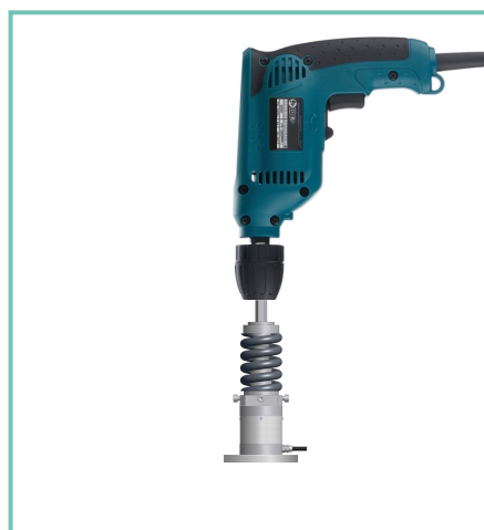
Torque measurement using fidaptor
